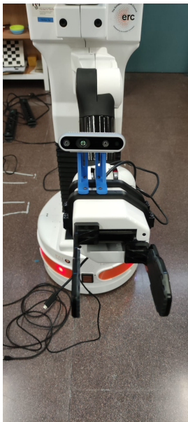
Fig. 2: Camera location based on the eye-in-hand configuration
