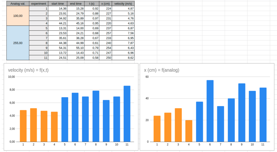
Fig. 13: Experimental results, throwing a ball several times
